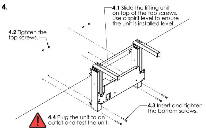
IMPORTANT NOTICE! While testing, keep hands and tools away from the open mechanism. Before continuing work, unplug the unit.
