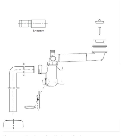
Place a vessel, such as a hand basin, under the water trap.
